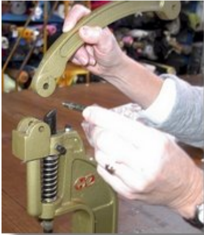
Locate the axle bolt, place handle in position.
