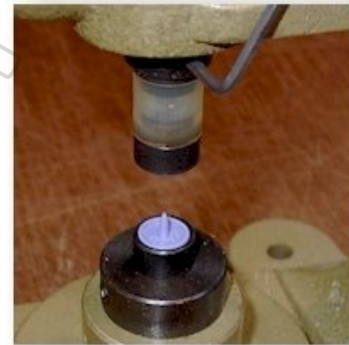
Slide the die up into the socket then gently tighten the set screw
