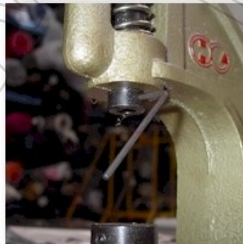
loosen the set screw on the arbor using supplied Allen key
